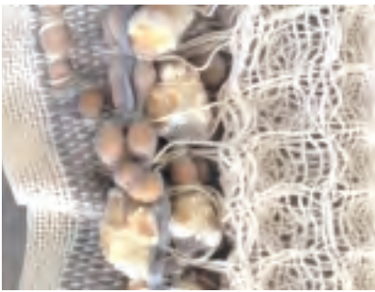
Figure 62: The cotton-corn weave after activation; the corn popped but remained in place.
