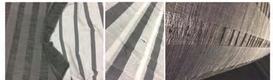
Figure 22 (Upper layer binding 2/2 for creating an open construction, more dense construction 1/1 on the backside. Both layers are joined using a 2x4 construction.)
