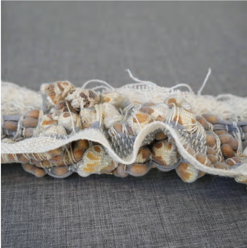
Figure 56: The activated cloth after it had been heated in a microwave oven.
