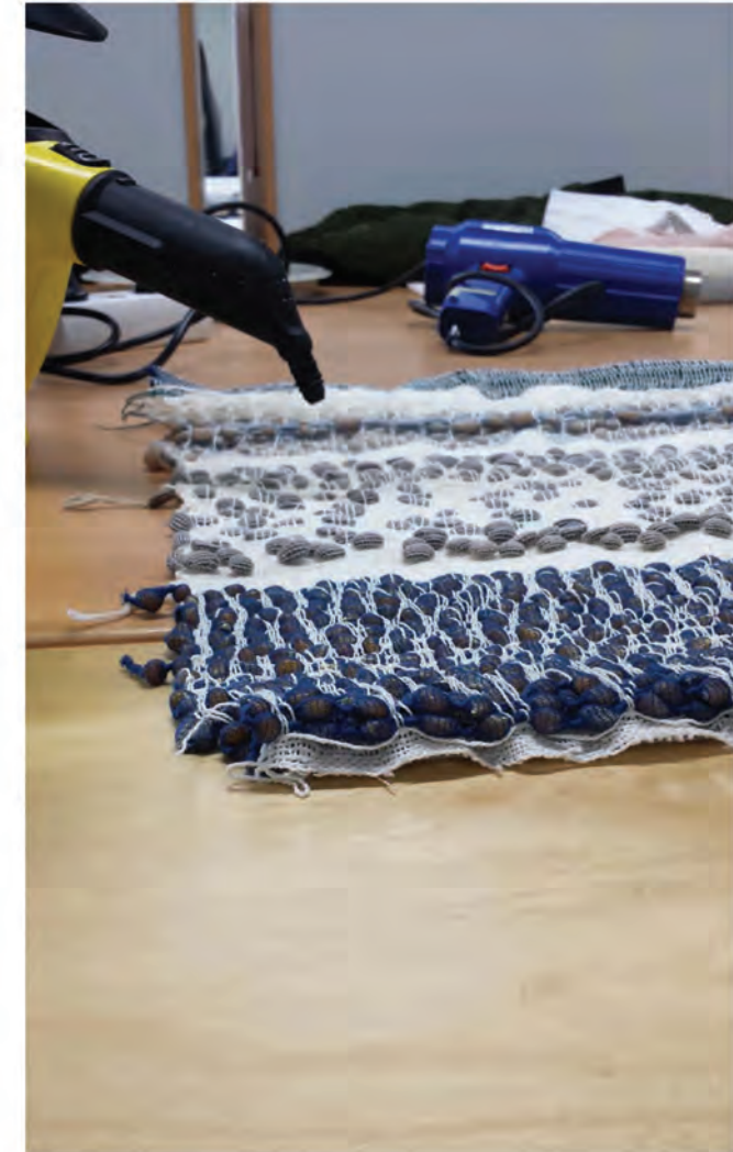
Figure 5. Activating fabric with water
