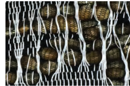
Figure 43: A textile-seed yarn that was used as a weft material.
