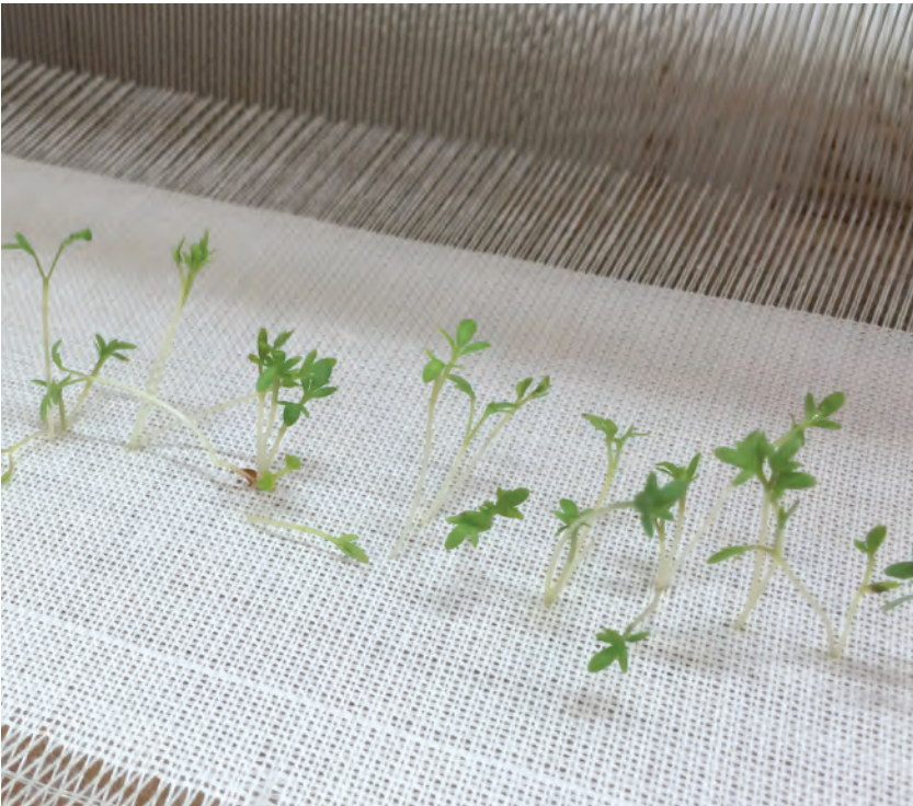
2 Day 0 Figure 88: The cress seedlings were integrated in the process of weaving with a PVA yarn on a shaft loom with a cotton warp.
