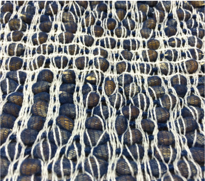
1 Figure 49: The cotton-corn yarn, which was used as a weft material. The warp material, an off-white wool yarn, was also used as additional weft (shown in the upper part of the image).
