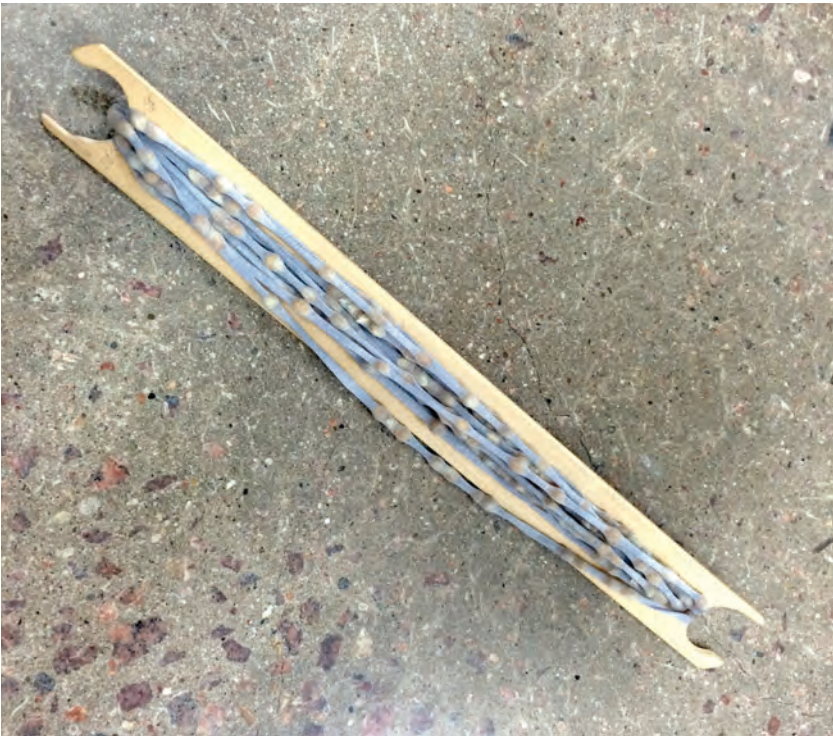
Figure 59: The cotton-corn yarn on the weaving shuttle.
