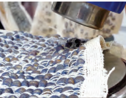
Figure 55: Another method of activating the corn was to use a heat gun.
