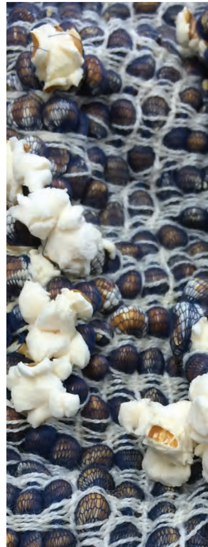
3 Min 5 Figure 54: The popped corn damaged the tubular knit and partially or entirely became detached from it.
