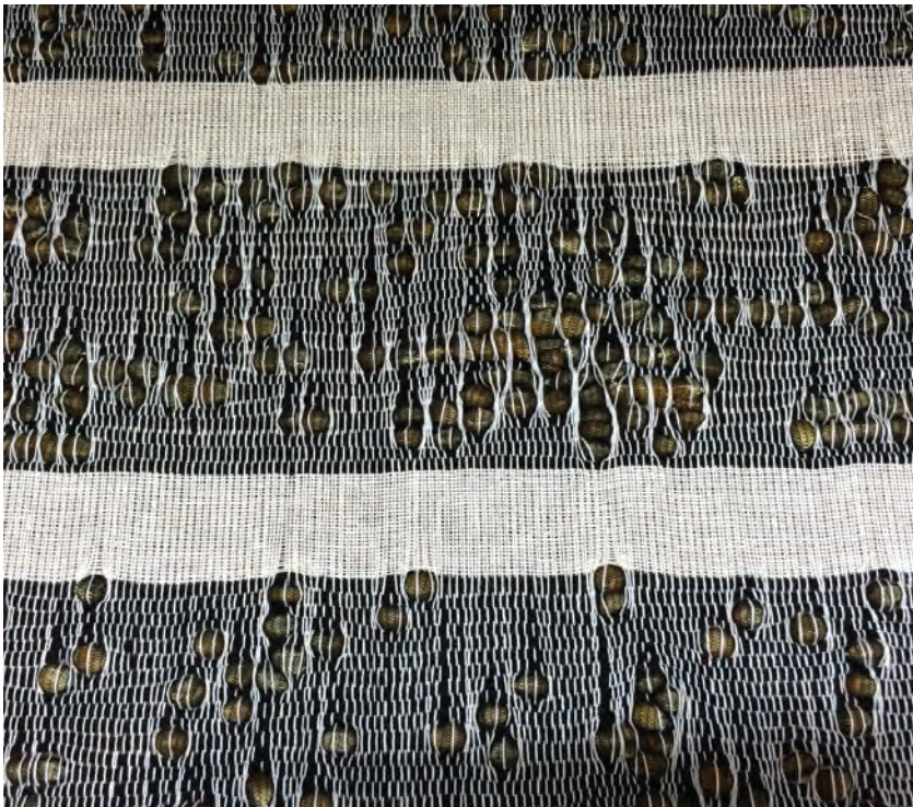
Figure 68: The random pattern that appeared when the black cotton corn yarn was woven with a plain weave. The white stripes separated the different sections.
